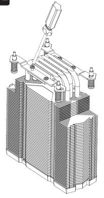
Install the bracket mount on the cooler base. Fasten the bracket mount with screws
