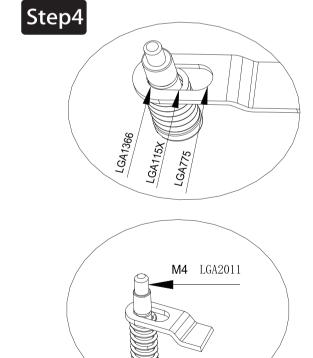
Move the screw on the bracket to the corresponding position according to the main board type. (As shown in the above figure)
