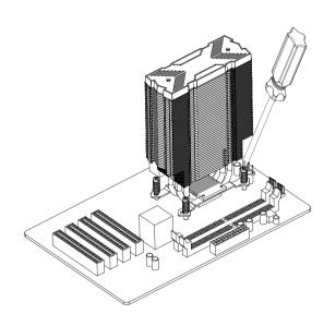
Place the radiator on the CPU and screw the bracket screw to the base of the original cooling rack (Pictured above)
