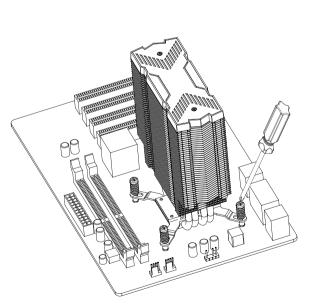
Place the radiator on the CPU while aligning the support screw to the backplane nut and tightening (Pictured above)
