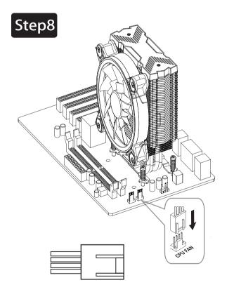
EN After installing the fan, connect the fan wire to the main board
