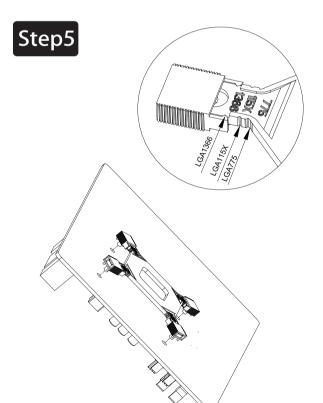
The backplane positioning slider is moved to the desired position and loaded into the main board. If your motherboard is Iga2011, use the original motherboard backplane.
