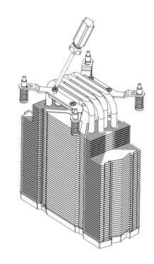
Install the bracket mount on the cooler base. Fasten the bracket mount with screws.
