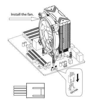
**EN** After installing the fan, connect the fan wire to the main board
