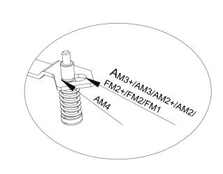
Move the screw on the bracket to the corresponding position according to the main board type. (As shown in the above figure)
