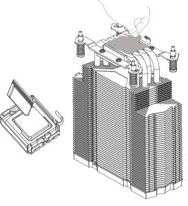
EN Evenly spread the heat sink paste on the surface of the CPU and remove the bottom of the radiator.
