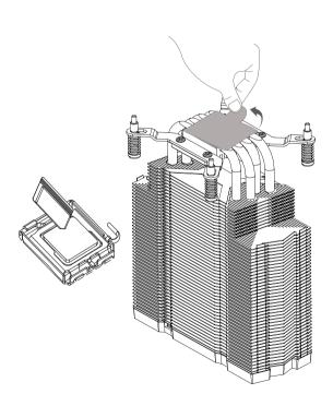
**EN** Evenly spread the heat sink paste on the surface of the CPU and remove the bottom of the radiator.
