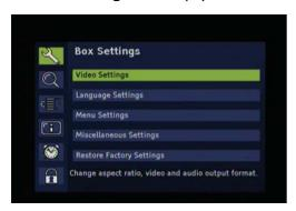
By using the **arrow keys** ▲ or ▼, highlight the desired option and press the **OK key** in order to call it up.
