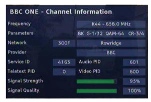
4 Adjust your antenna so that the two specifications signal strength and signal quality display a preferably high value.
