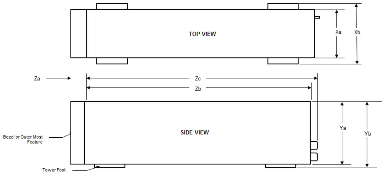
Figure 3. Chassis dimensions
