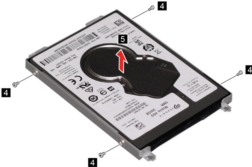
Figure 25. Remove four screws and remove the storage drive
