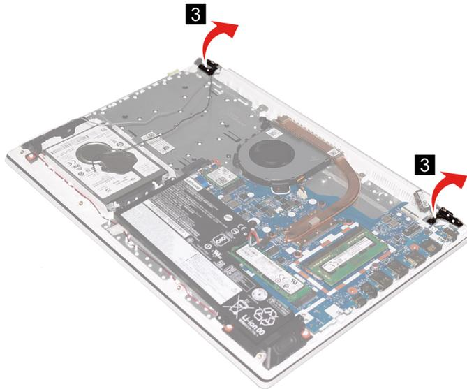
Figure 34. Open the hinges
