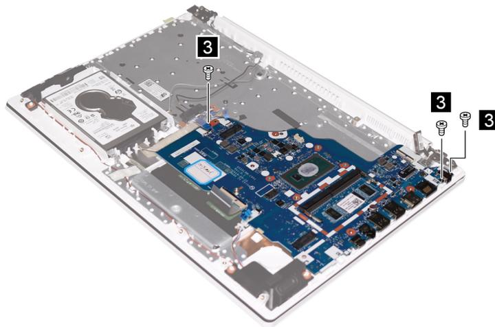
Figure 30. Remove three screws
