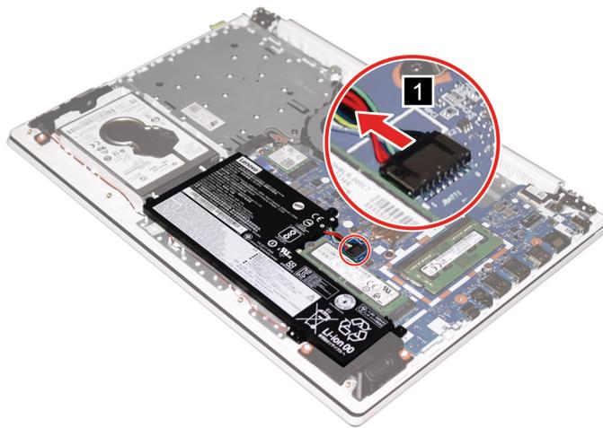
Figure 20. Remove the battery pack cable
