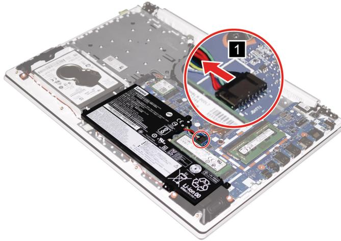
Figure 22. Remove the battery pack cable
