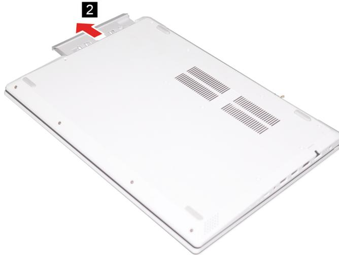
Figure 3. Remove the ODD
