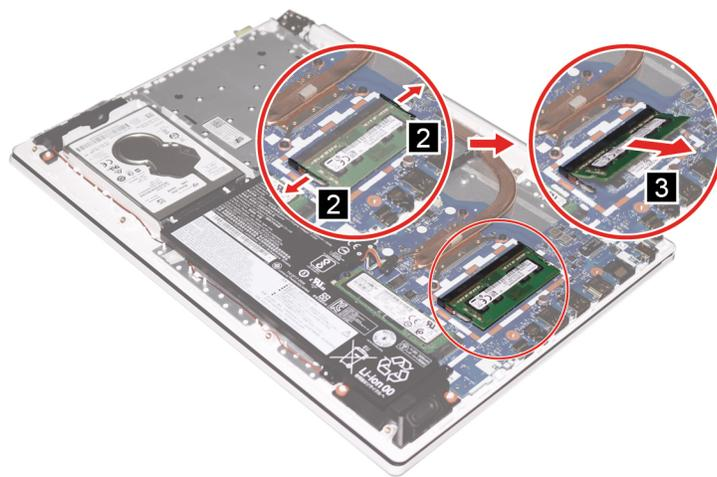
Figure 11. Press the clips and slide the memory module out of the slot
