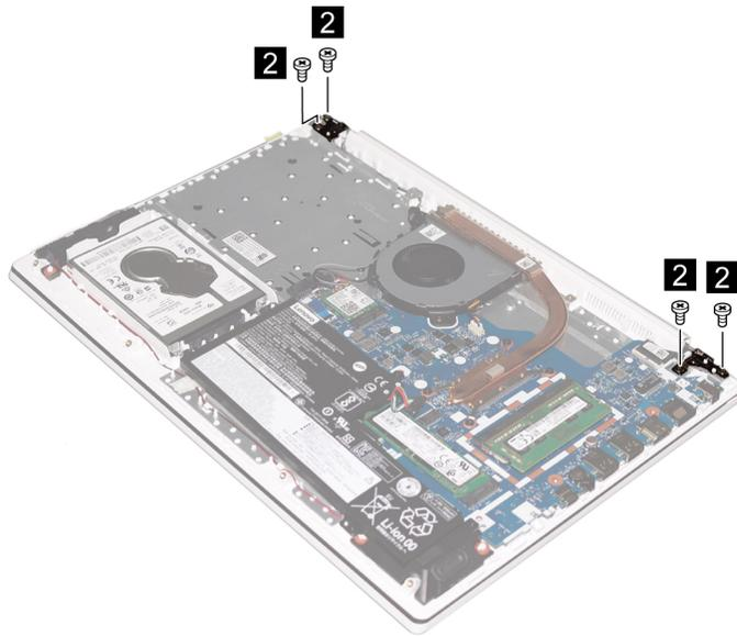
Figure 33. Remove four screws
