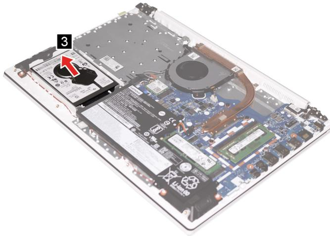
Figure 24. Remove the storage drive with bracket
