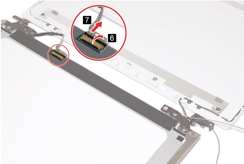
Figure 40. Disconnect the EDP cable
