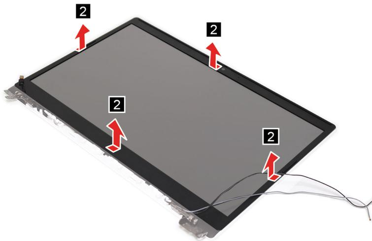
Figure 37. Remove the LCD bezel
