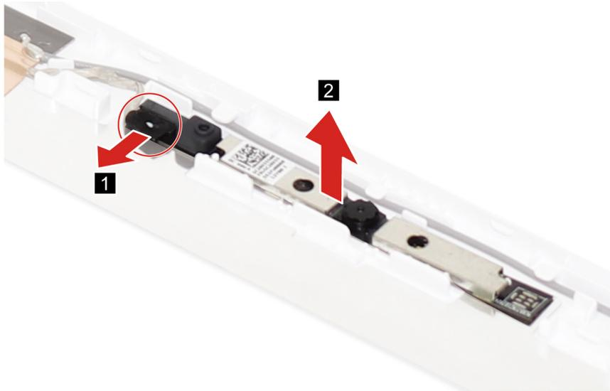
Figure 43. Disconnect the camera module cable and remove the camera module
