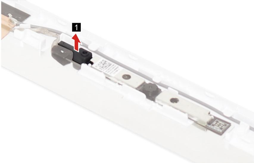
Figure 42. Remove the microphone rubber
