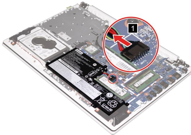
Figure 26. Remove the battery pack cable
