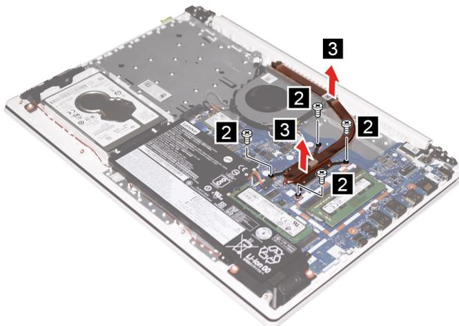
Figure 15. Loosen four screws and remove the heat sink
