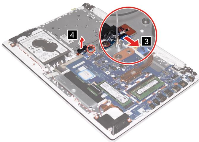
Figure 28. Disconnect the cable from the system board and remove the ODD board
