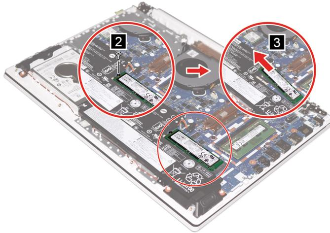
Figure 9. Remove one screw and slide the M.2 solid-state drive out of the slot
