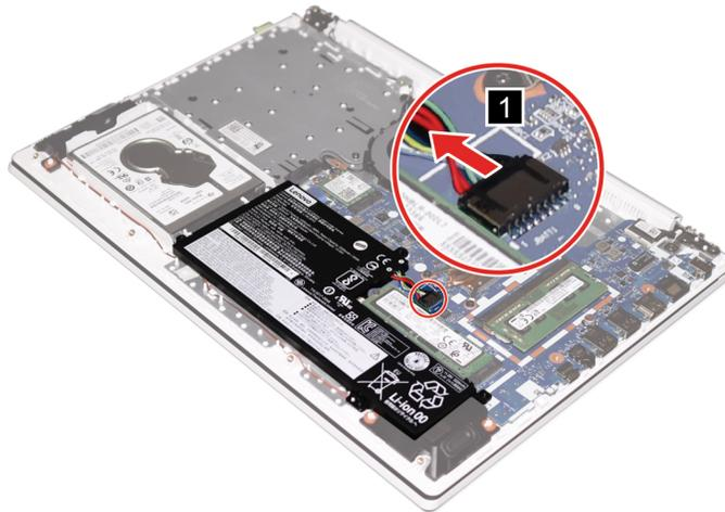
*Figure 8. Remove the battery pack cable*
