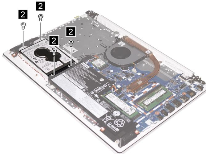
Figure 23. Remove four screws
