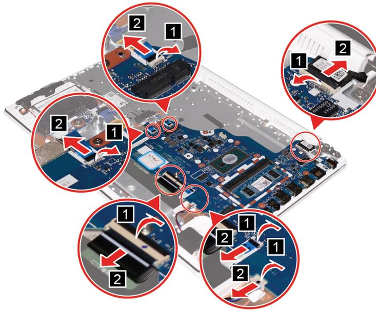
Figure 29. Disconnect cables
