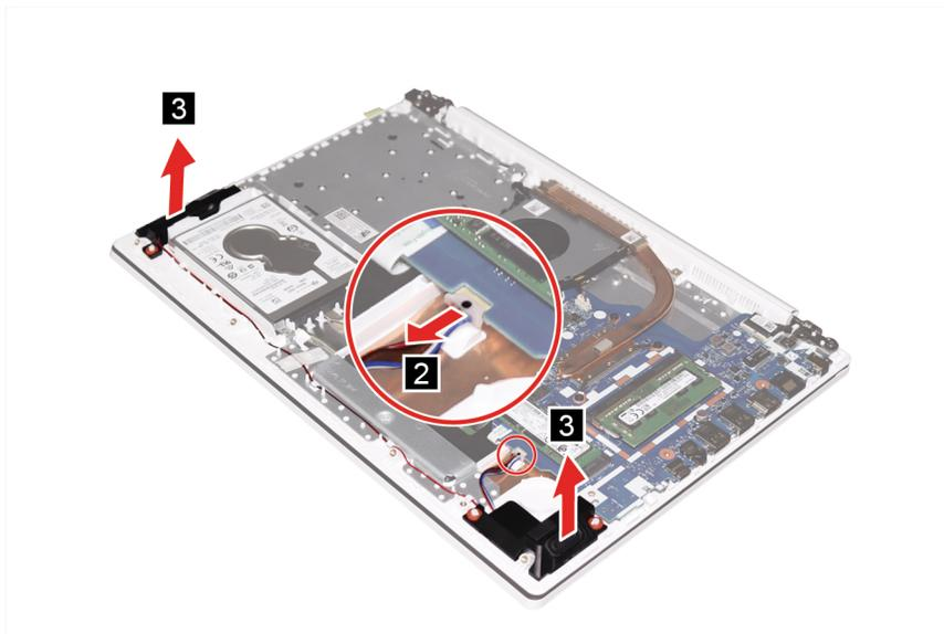
Figure 21. Disconnect the speaker cable and carefully remove the speakers
