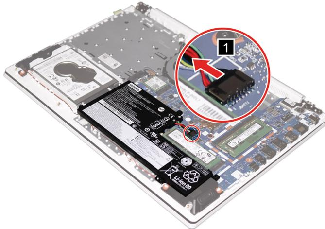
Figure 6. Remove the battery pack cable
