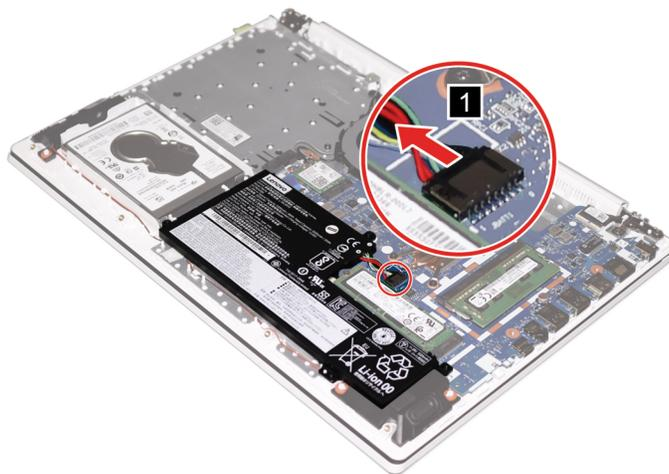
Figure 16. Remove the battery pack cable
