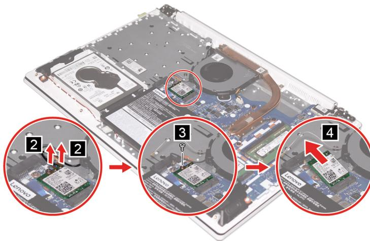
Figure 13. Remove one screw and slide the Wi-Fi card out of the slot
