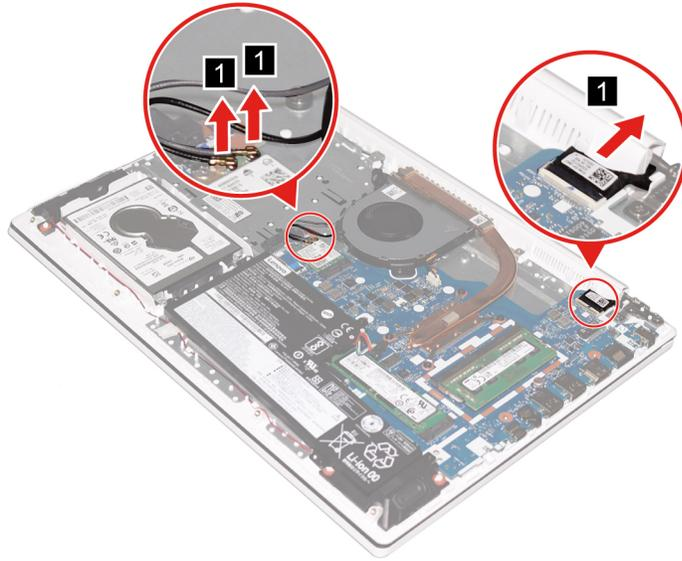
Figure 32. Disconnect the WLAN cables and the EDP cable
