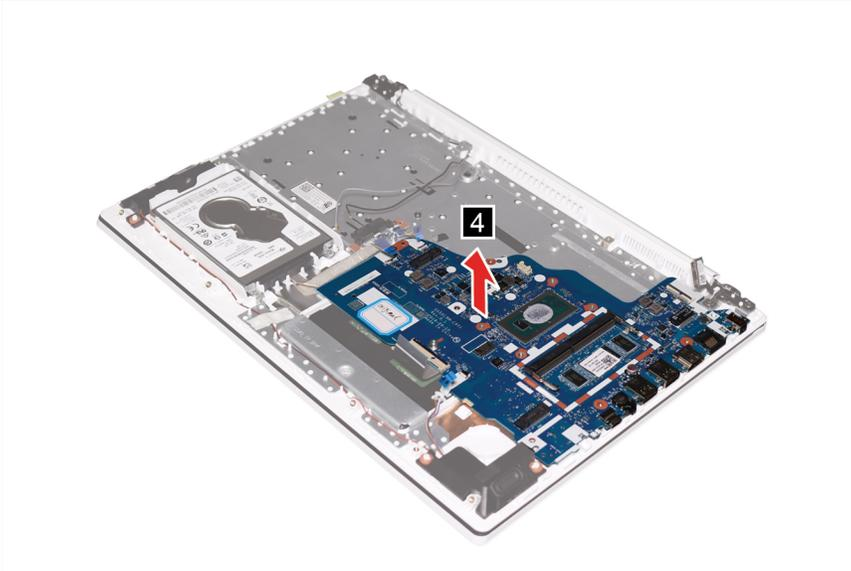
Figure 31. Remove the system board
