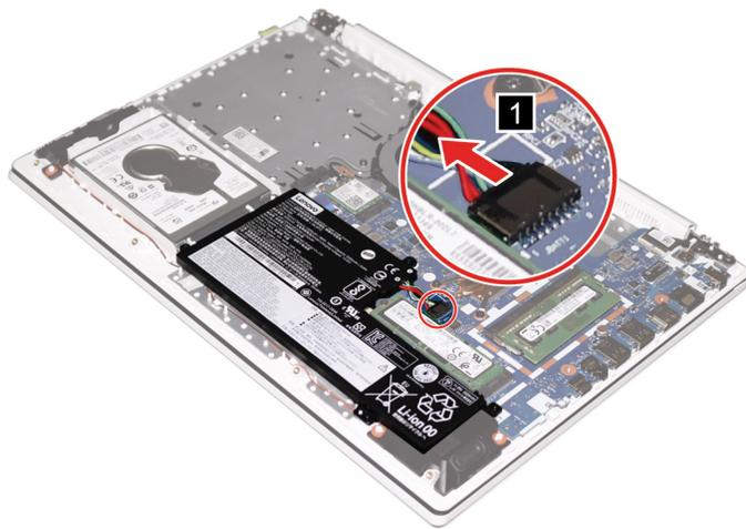
Figure 10. Disconnect the battery pack cable
