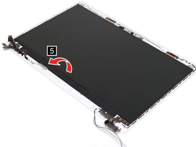
Figure 39. Carefully lift the LCD panel from the LCD cover
