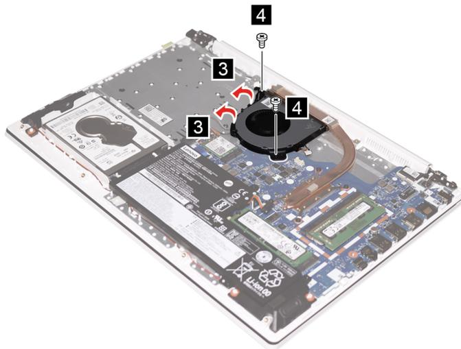
Figure 18. Remove the fan cables from the hooks and then remove two screws
