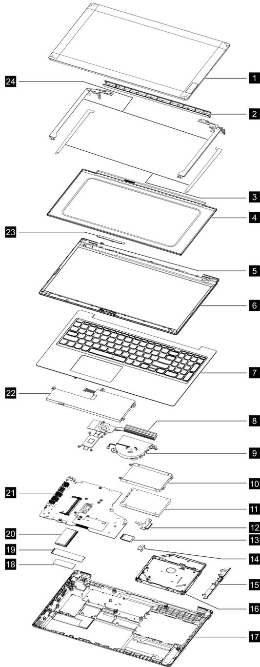
Figure 1. IdeaPad L3 15IML05, IdeaPad L3 15IML05 U, and IdeaPad L3 15IML05 D exploded view
