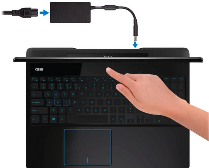
**NOTE:** To conserve battery power, the battery might enter power saving mode. Connect the power adapter and press the power button to turn on the computer.
