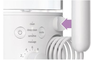
When the patient is finished, they can simply return the handle to the easy magnetic dock. The handle automatically switches from pause to off.
