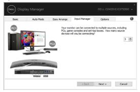
In PC1-PC3, select the Video Input Port to connected to the port and select the USB Upstream Port to connected to the port, then press NEXT.
