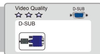
**Step 2:** Connect video signal with appropriate connector cable.
