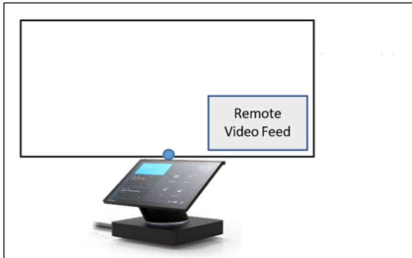
When the RXV100Hub is connected to a single external screen, both remote participants and remote content share the screen space. When two external screen are connected to the RXV100Hub, an optional setting allows the screens to be swapped (the remote video feed and the content feed).
