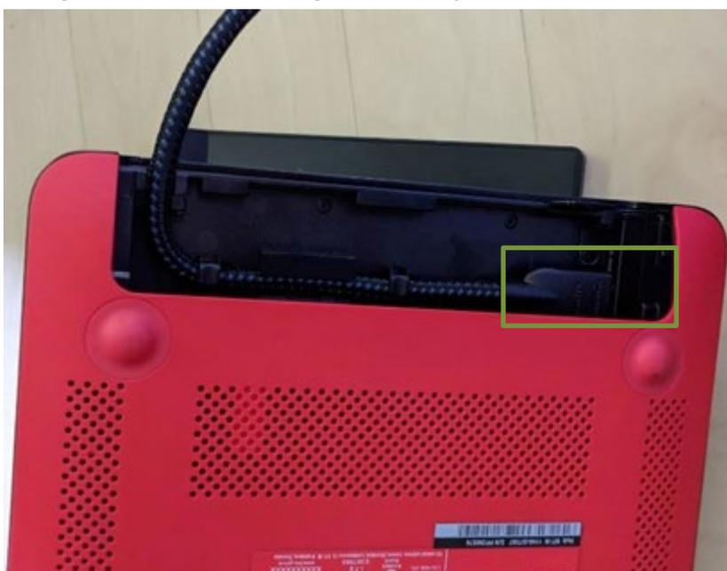
3. On the red side of the One Cable, slide the plastic cover down to reveal the block of connectors.
