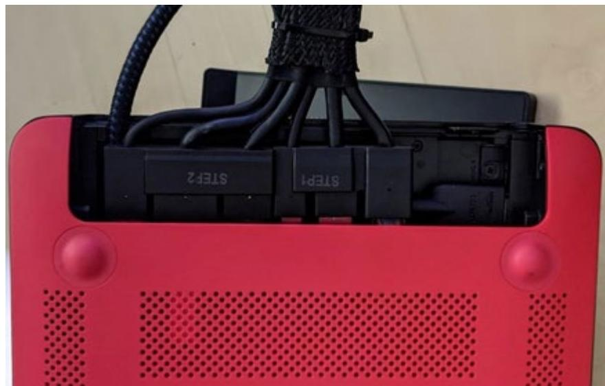
5. Keeping the device on its side with the ports/cables facing up, slide the red cover along One Cable, align the HDMI ingest cable to the notch and snap the cover into place. You may find it easier to hold the cables in one hand while sliding the cover with the other hand.
