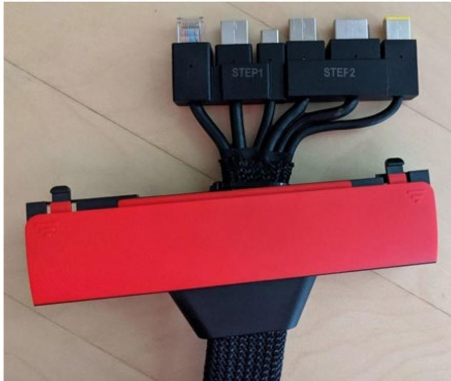
4. Align the connectors labeled 'Step 1' and 'Step 2' to the ports on the base shown in the figure below. Gently push the connectors into the corresponding ports, moving from right to left.
