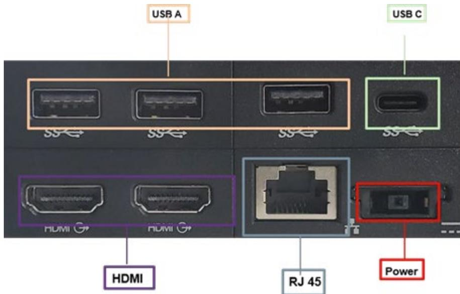
2. Ensure the HDMI cable is not faulty or loose
