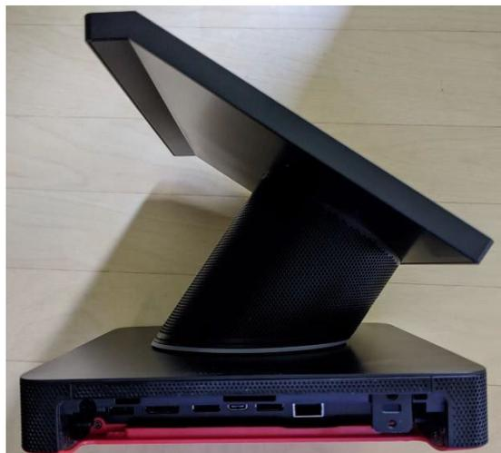
2. Insert an HDMI cable into the HDMI ingest port on the inner right sidewall of the base shown in the figure below, lace it through the security channel and set it into the rounded notch.
