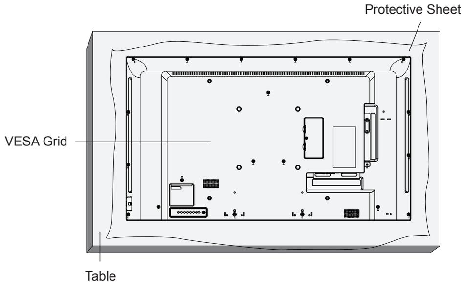
1. Lay a protective sheet on a table, which was wrapped around the display when it was packaged, beneath the screen surface so as not to scratch the screen face.
