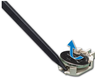
Figure 120. Removing the system battery
