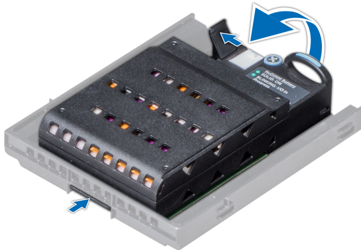
Figure 43. Removing NVDIMM-N battery from the bracket
