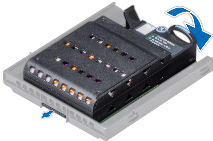
Figure 44. Installing NVDIMM-N battery into the bracket
