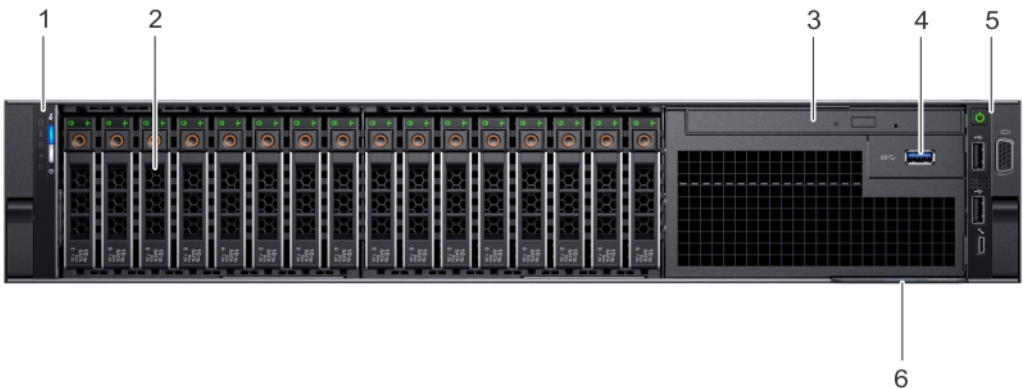
Figure 2. Front view of 16 x 2.5 inch drive system
