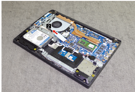
Figure 10. Remove the SSD
