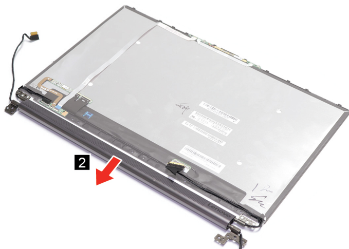
Figure 40. Remove the hinge and soundbar module
