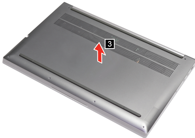
Figure 4. Remove the lower case
