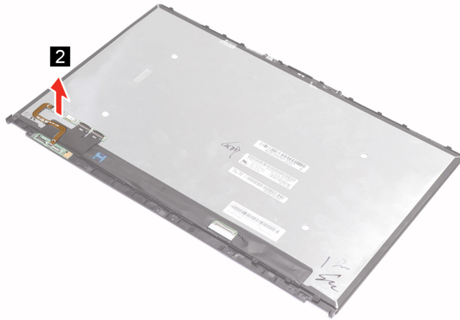
Figure 44. Remove the trans board
