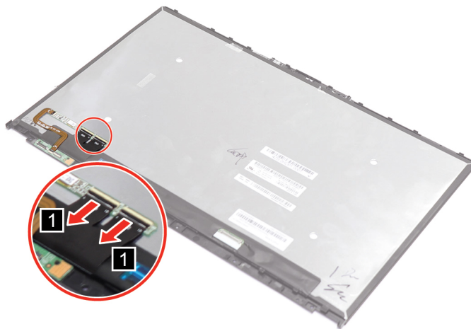
Figure 43. Disconnect the cables
