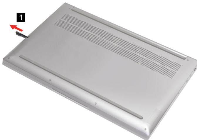
Figure 2. Pull the active pen out of the slot
