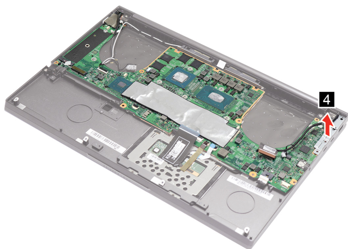
Figure 24. Remove I/O bracket
