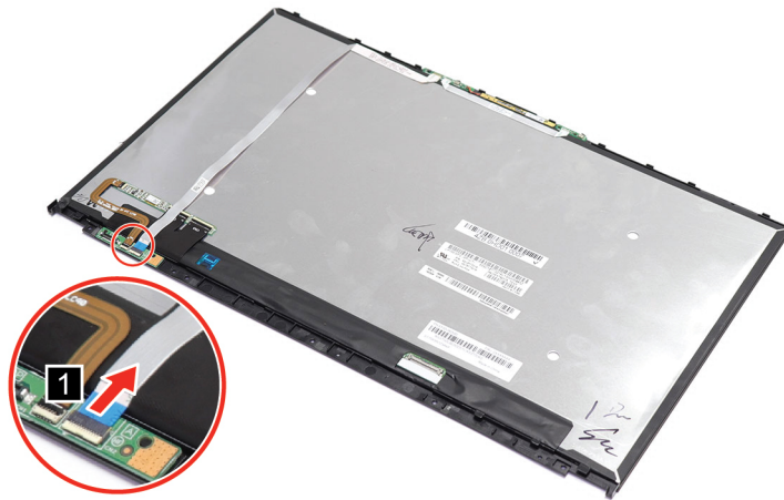
Figure 41. Disconnect the cable
