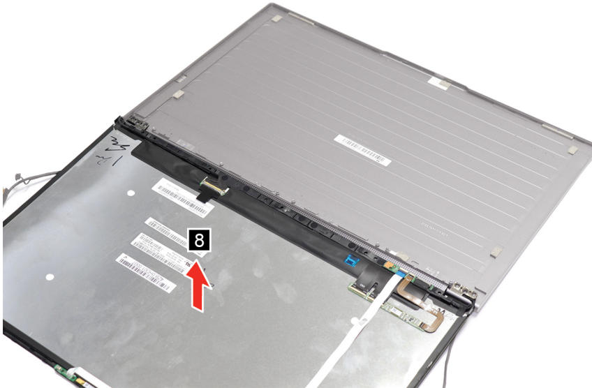
Figure 38. Remove the LCD panel
