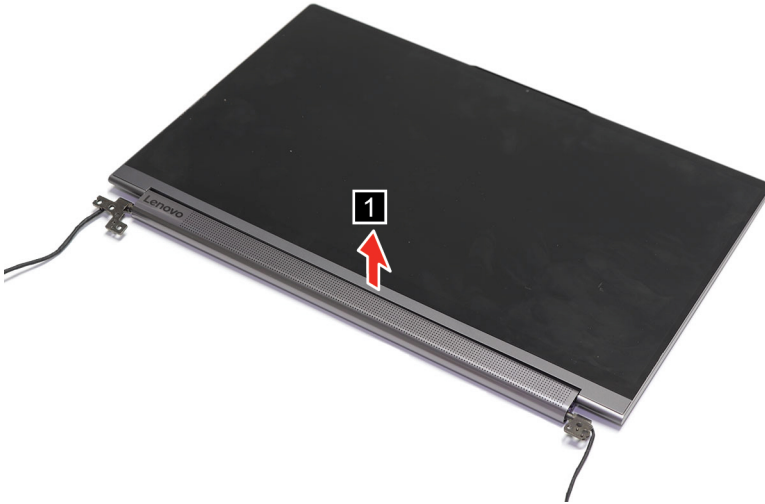
Figure 34. Remove the bezel tape
