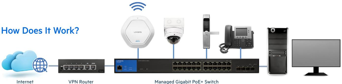
Linksys Managed Gigabit PoE+ switches can power PoE+ enabled devices such as surveillance cameras, access points, door access control systems, VoIP phones and ProAV systems. This will eliminate the need for additional power cables and outlets, making installation simpler and less expensive.
