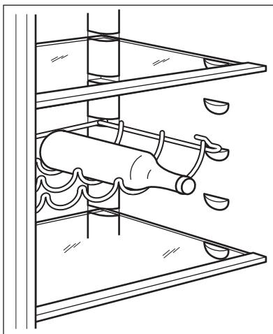
2. This shelf can be tilted to store unsealed bottles. To obtain this result, place front hooks of the shelf one level higher than the rear hooks.
