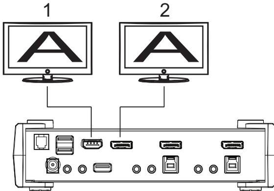
With an external MST hub (not included) you can copy video content to one HDMI and two DisplayPort monitors, as shown below.
