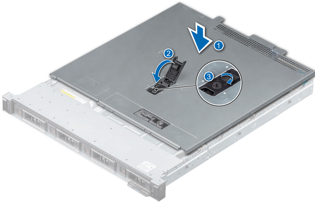
Figure 12. Installing the system cover
