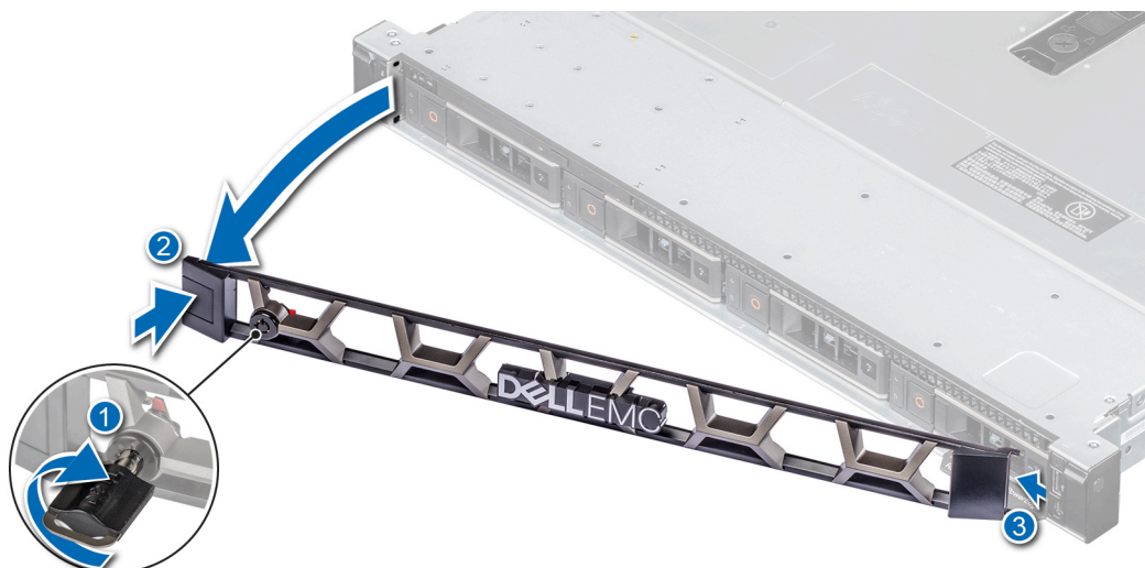
Figure 9. Removing the front bezel
