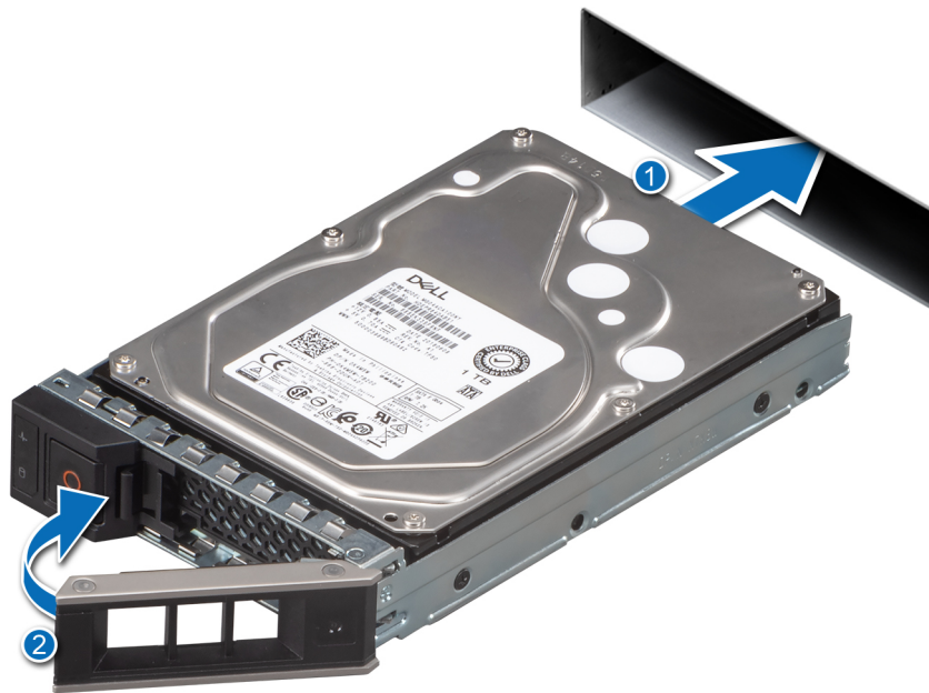
Figure 22. Installing the hot-swappable drive
