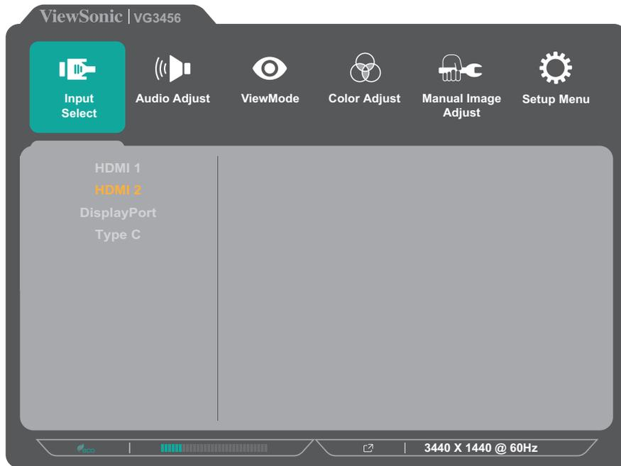
3. Press the **1 (ViewMode)** or **2** key to select the desired input source. Then press the **3** key to confirm the selection.
