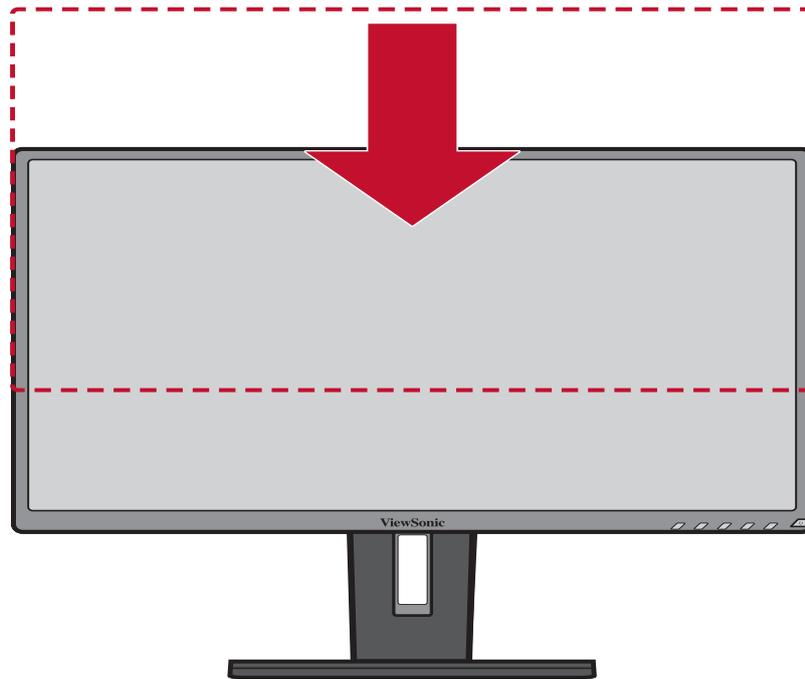
**NOTE:** When adjusting, press down firmly along the adjustment track.
