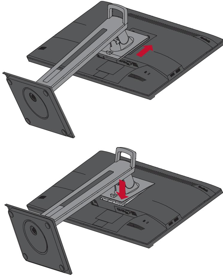
**NOTE:** Ensure the stand is secure and the quick release tab positively clicks into place.
