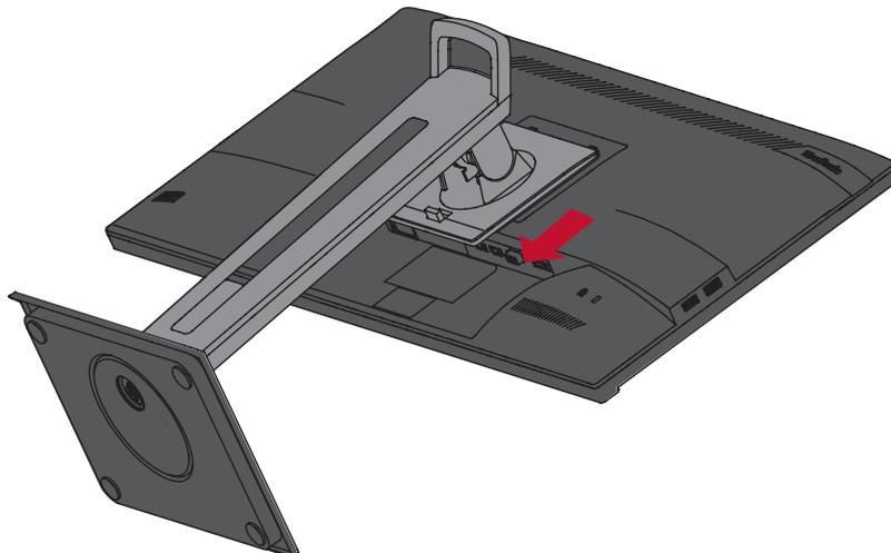
5. Attach the mounting bracket to the VESA mounting holes at the rear of the device. Then secure it with four (4) screws (M4 x 10 mm).
