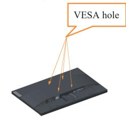
Step 5: Attach the LCD display to the wall, and follow the instructions in the wall-mounting kit. For use only with UL Listed Wall Mount Bracket with minimum weight/load: 8kg
