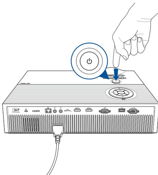
2. When the following screen appears, press the power button again to completely turn off your LED projector.
