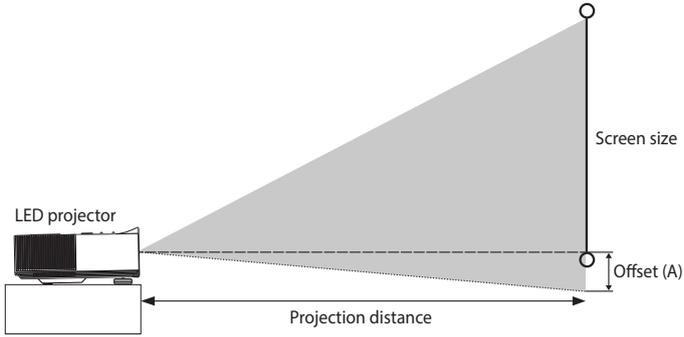
**NOTE:** The screen aspect ratio is 16:9 (1920 x 1080) and the projected image is in a 16:9 aspect ratio.
