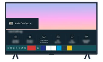
Check the volume on the screen. If a number for the TV volume is not displayed, select (a) > (b) Sound Output. Then, select TV Speaker.
