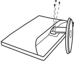
2. Remove the 3 screws and then remove the base from the monitor.
