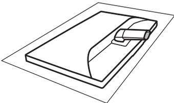
2. Hold the monitor base stand with both hands and firmly insert the base stand into the base column.
