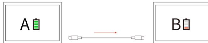
**Note:** The remaining battery power of computer A should be at least 30% and be 3% higher than that of computer B.
