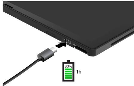
**Note:** To maximize the life of the battery, use the battery until the charge is depleted and recharge the battery completely before using it. Once the battery is fully charged, it must discharge to 94% or lower before it will be allowed to recharge again.
