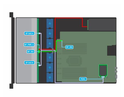
Figure 40. Cable routing -  $8 \times 3.5$  inch drive backplane with mini PERC card
