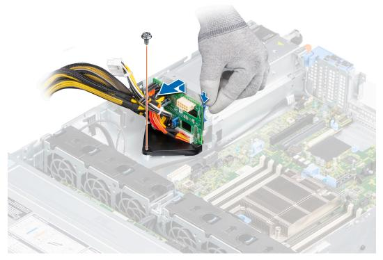
Figure 122. Removing the power interposer board
