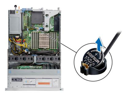
Figure 110. Removing the system battery
