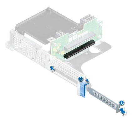
Figure 79. Installing a filler bracket for riser 1B
