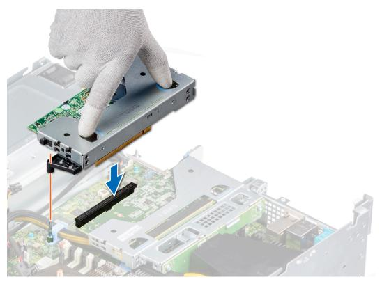
Figure 69. Installing the riser 2
