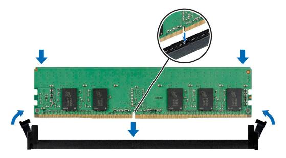
Figure 56. Installing a memory module
