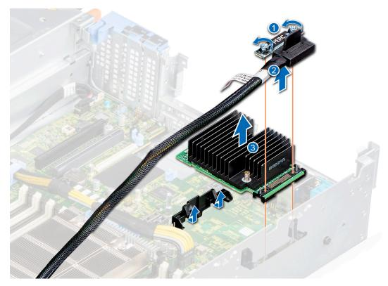
Figure 108. Removing the Internal mini PERC card
