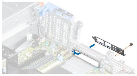
Figure 104. Installing the LOM riser bracket
