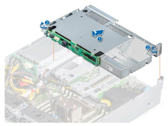
Figure 54. Installing the rear drive cage
