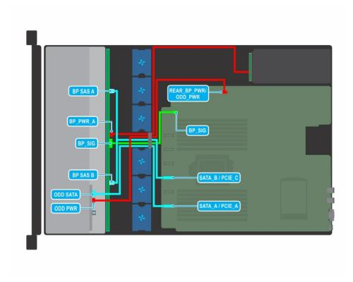
Figure 39. Cable routing - 8 x 3.5 inch drive backplane with ODD
