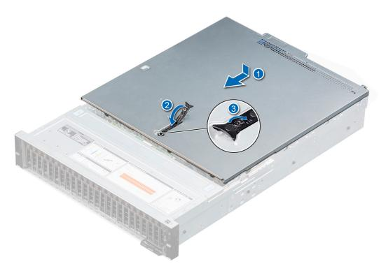
Figure 20. Installing the system cover
