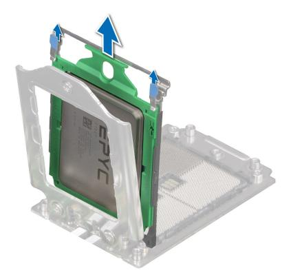
Figure 60. Removing the processor tray
