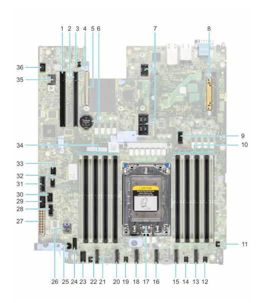
Figure 131. System board connectors
