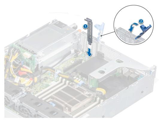
Figure 73. Installing the filler bracket
