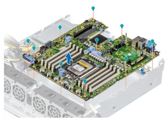
Figure 124. Removing the system board
