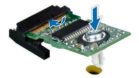
Figure 126. Installing the TPM
