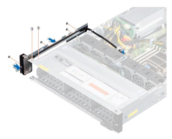
Figure 128. Installing the left control panel
