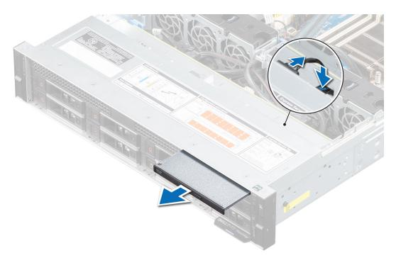
Figure 114. Removing optical drive
