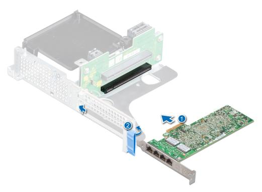
Figure 85. Installing the expansion card into a riser 1B
