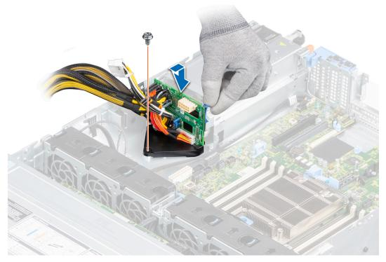
Figure 123. Installing the power interposer board
