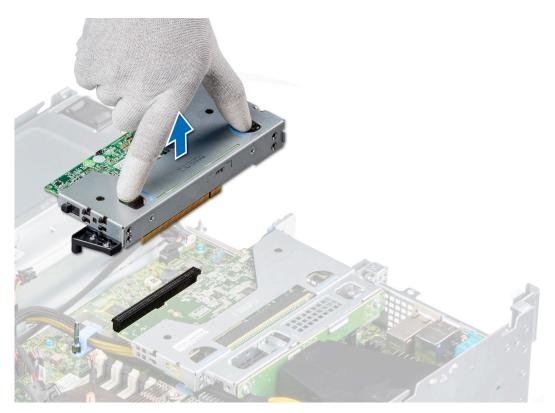
Figure 66. Removing the riser 2
