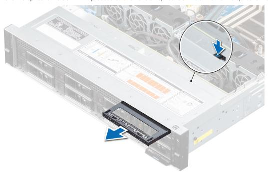
Figure 116. Removing optical blank
