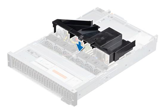
Figure 26. Installing the air shroud for system with rear drives
