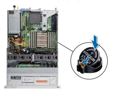
Figure 111. Installing the system battery
