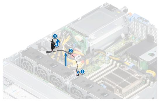
Figure 31. Removing the intrusion switch
