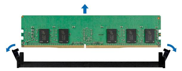
Figure 55. Removing a memory module
