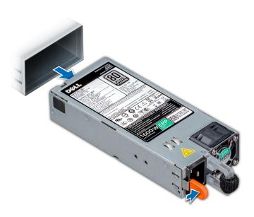
Figure 119. Removing a power supply unit
