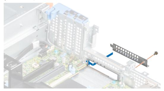
Figure 102. Installing the LOM filler bracket
