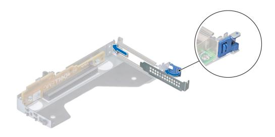
Figure 81. Installing a filler bracket for riser 2
