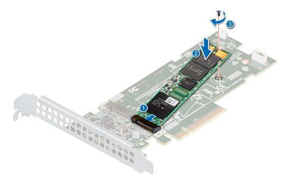
Figure 95. Installing the M.2 SSD module
