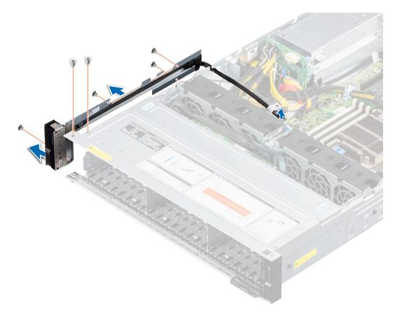
Figure 127. Removing the left control panel
