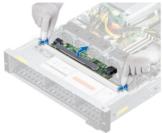
Figure 49. Removing the drive backplane
