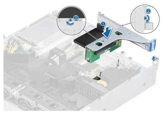
Figure 71. Installing the riser 1B
