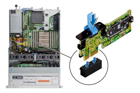
Figure 97. Installing IDSDM card
