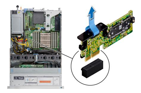
Figure 96. Removing the IDSDM card
