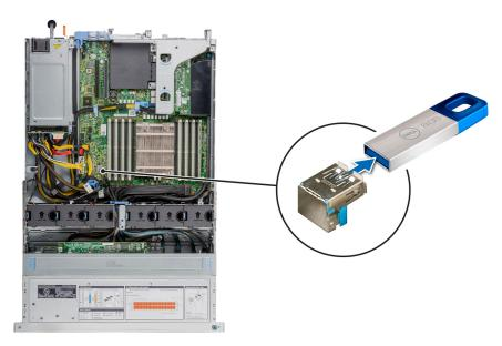
Figure 112. Removing the internal USB memory key
