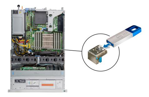
Figure 113. Installing the internal USB memory key
