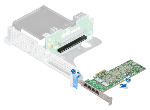
Figure 76. Removing the expansion card from riser 1B
