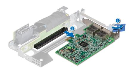
Figure 77. Removing the expansion card from riser 1A
