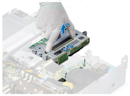
Figure 67. Removing the riser 1A
