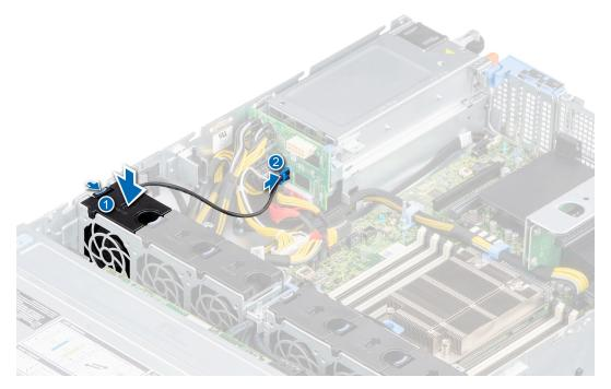
Figure 30. Connecting fan 1 cable to PIB
