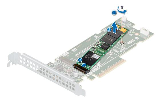
Figure 94. Removing the M.2 SSD module
