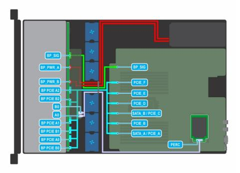
Figure 42. Cable routing -  $12 \times 2.5$  inch SAS drive +  $12 \times 2.5$  inch NVMe drive backplane
