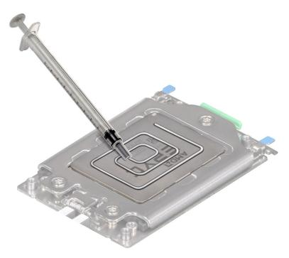
Figure 64. Applying thermal grease on the processor
