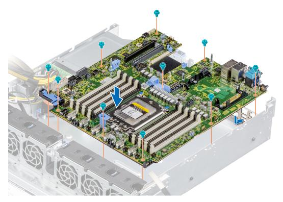
Figure 125. Installing the system board
