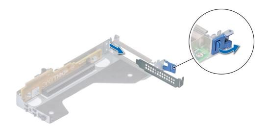
Figure 84. Removing a filler bracket for a riser 2
