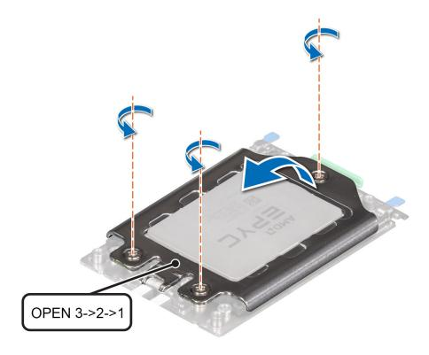
Figure 58. Removing screws on the force plate
