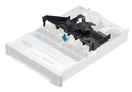
Figure 25. Installing the air shroud
