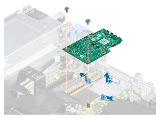
Figure 100. Removing the LOM riser card
