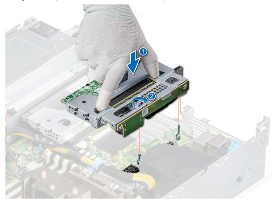
Figure 70. Installing the riser 1A
