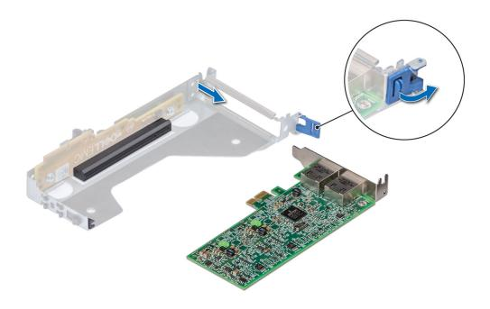
Figure 78. Removing the expansion card from riser 2
