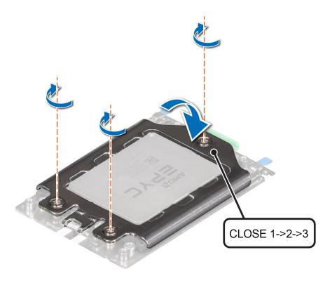
Figure 63. Securing the force plate
