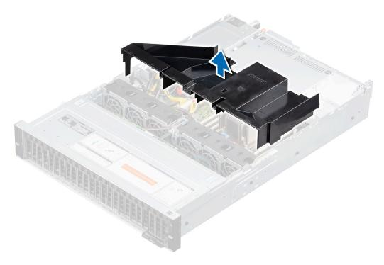
Figure 24. Removing the air shroud for system with rear drives
