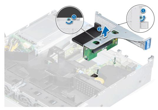
Figure 68. Removing the riser 1B
