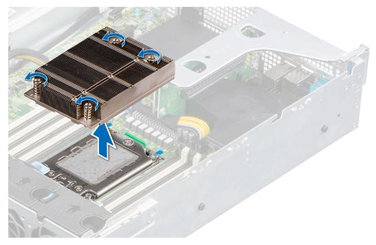
Figure 57. Removing the heat sink
