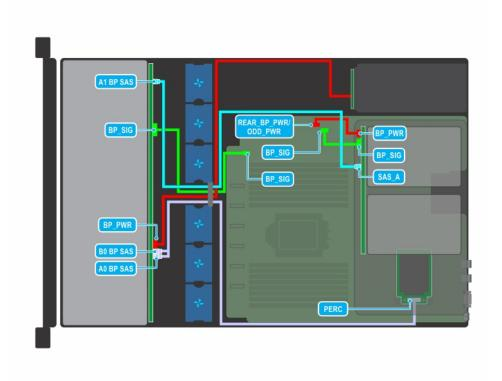
Figure 41. Cable routing -  $12 \times 3.5$  inch drive backplane with  $2 \times 3.5$  inch rear drive backplane
