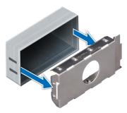
Figure 118. Removing a power supply unit blank
