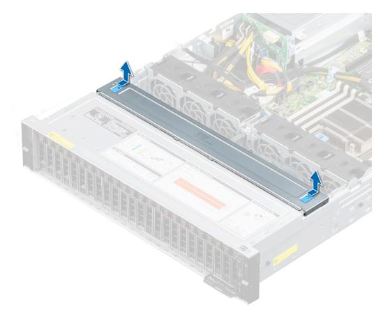
Figure 21. Removing the drive backplane cover
