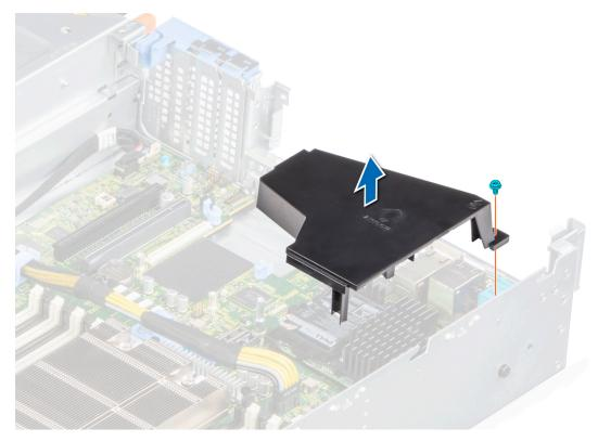
Figure 106. Removing the mini PERC card air shroud
