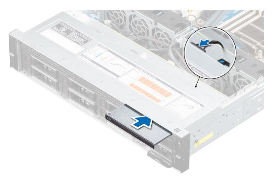
Figure 117. Installing optical drive
