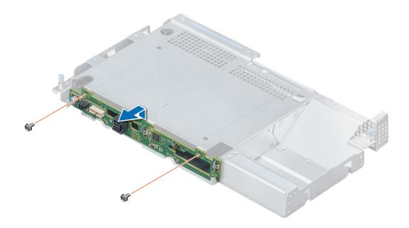
Figure 51. Removing the rear drive backplane
