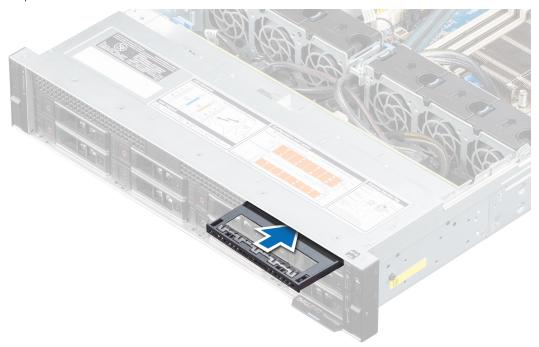
Figure 115. Installing optical drive blank
