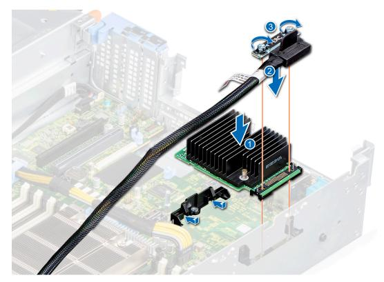
Figure 109. Installing the PERC card
