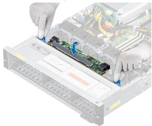
Figure 50. Installing the drive backplane
