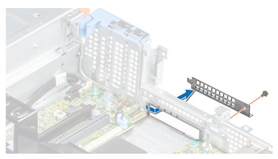
Figure 103. Removing the LOM filler bracket
