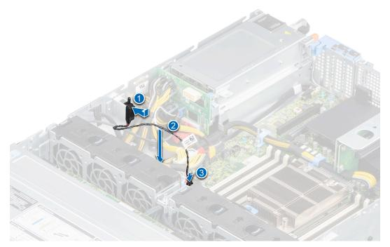
Figure 32. Installing the intrusion switch
