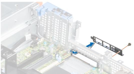
Figure 101. Removing the LOM riser bracket
