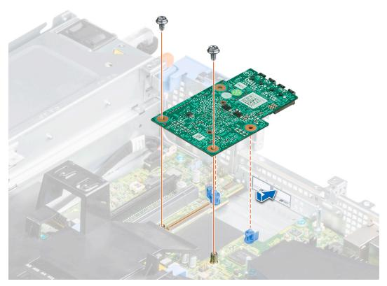
Figure 105. Installing the LOM riser card
