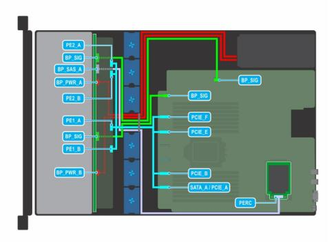
Figure 43. Cable routing - 24 x 2.5 inch NVMe drive backplane
