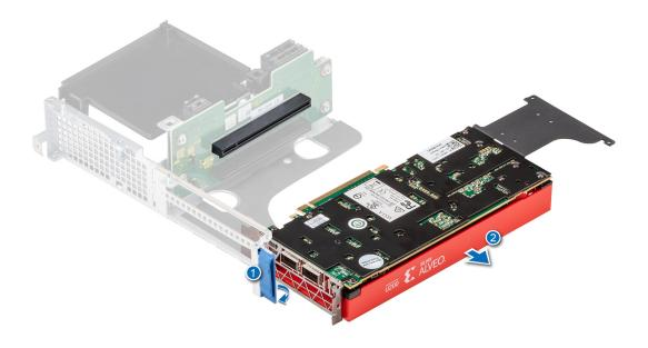
Figure 90. Removing the accelerator card from riser 1B
