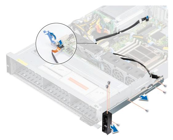
Figure 129. Removing the right control panel
