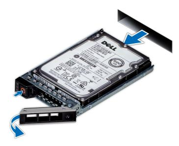
Figure 35. Removing the drive carrier
