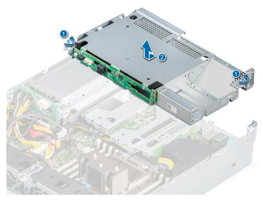
Figure 53. Removing the rear drive cage
