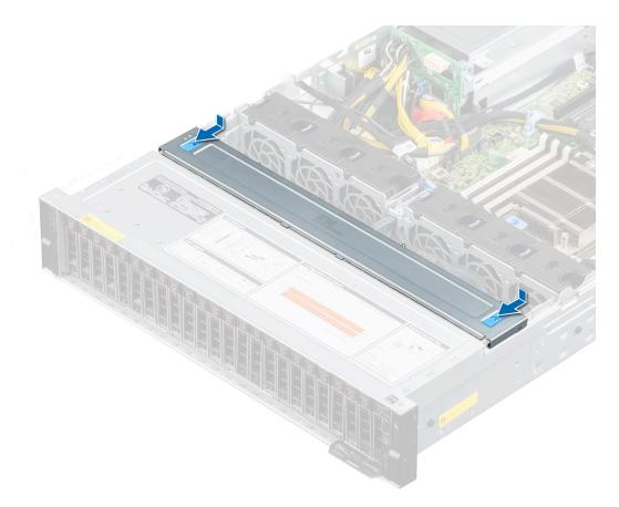
Figure 22. Installing the drive backplane cover
