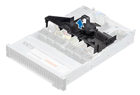
Figure 23. Removing the air shroud
