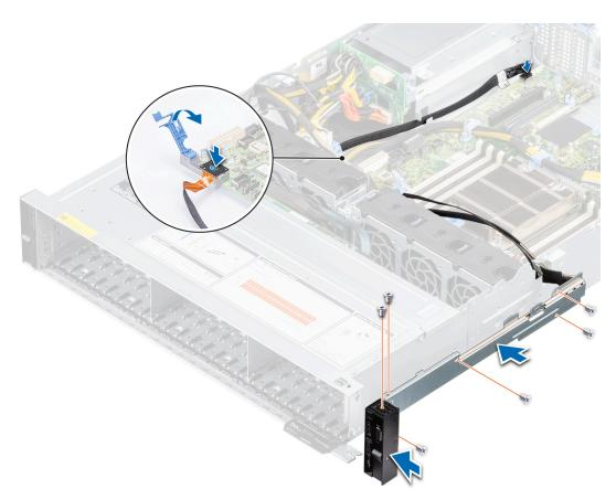
Figure 130. Installing the right control panel
