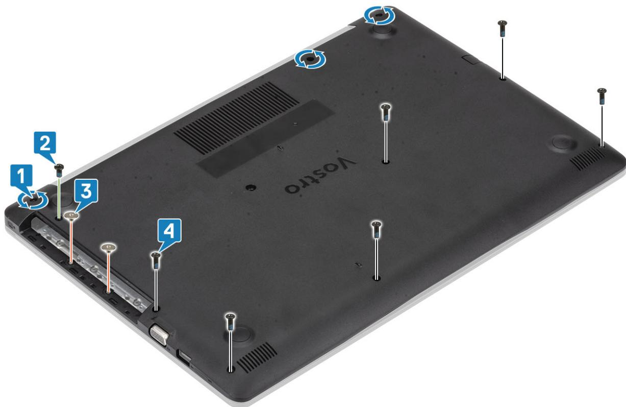
3. Pry the base cover from the top-right corner [1] and continue to open the right side of the base cover [2].
