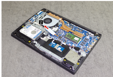
Figure 10. Remove the SSD
