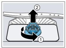
Pull down the micro filter to remove.
