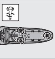
**7** Unscrew the 3 screws on the inside of the shaver and remove the back cover.
