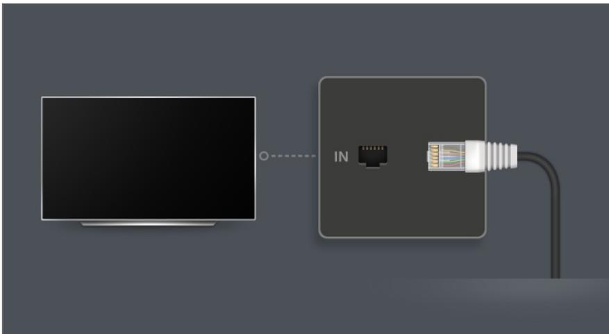
01 Connect the LAN port of the TV and the router using a LAN cable.
