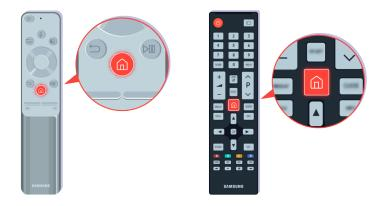
On the remote control, press the **a** button and move to **Settings** using the directional button.
