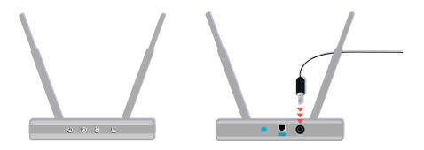
Make sure that your access point is working properly. If not, disconnecting and reconnecting the access point power cable may be required.
