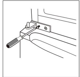
11. Place the upper door back on. Ensure the door is aligned horizontally and vertically so that the seal are closed on all sides before finally tightening the top hinge. Then insert the hinge and screw it to the top of the unit.
