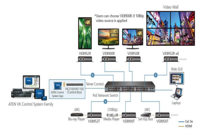
\*Note: VE8952 supports PoE and can be installed in combination with PoE network switches to reduce power cabling and additional power outlets. Before choosing the Network switch and installation, please refer to the Implementation Guide.
