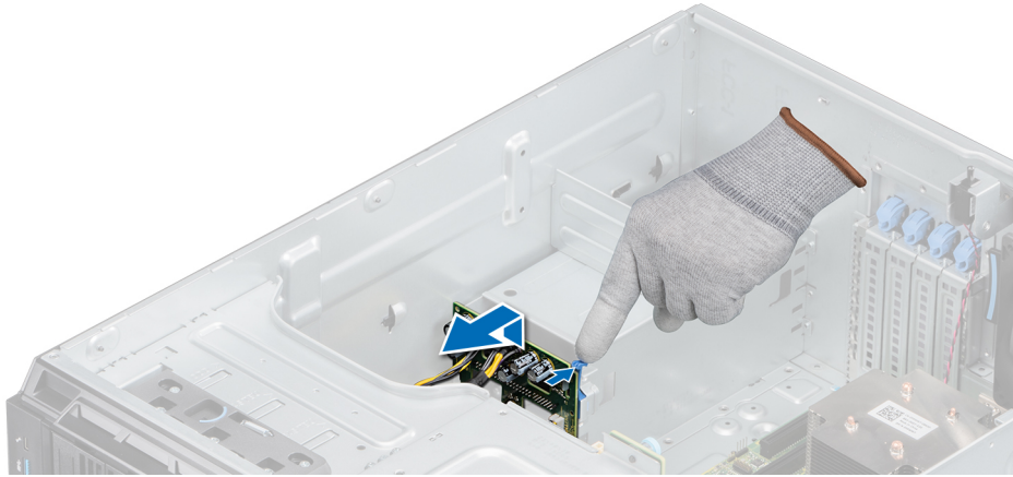
Figure 76. Removing the power interposer board
