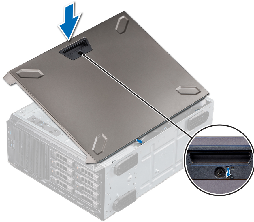
Figure 23. Installing the system cover
