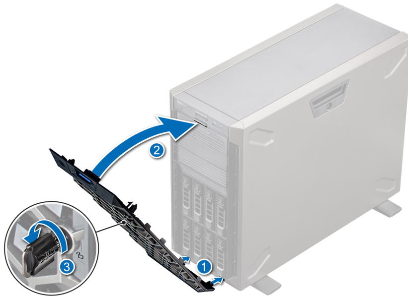
Figure 18. Installing the front bezel
