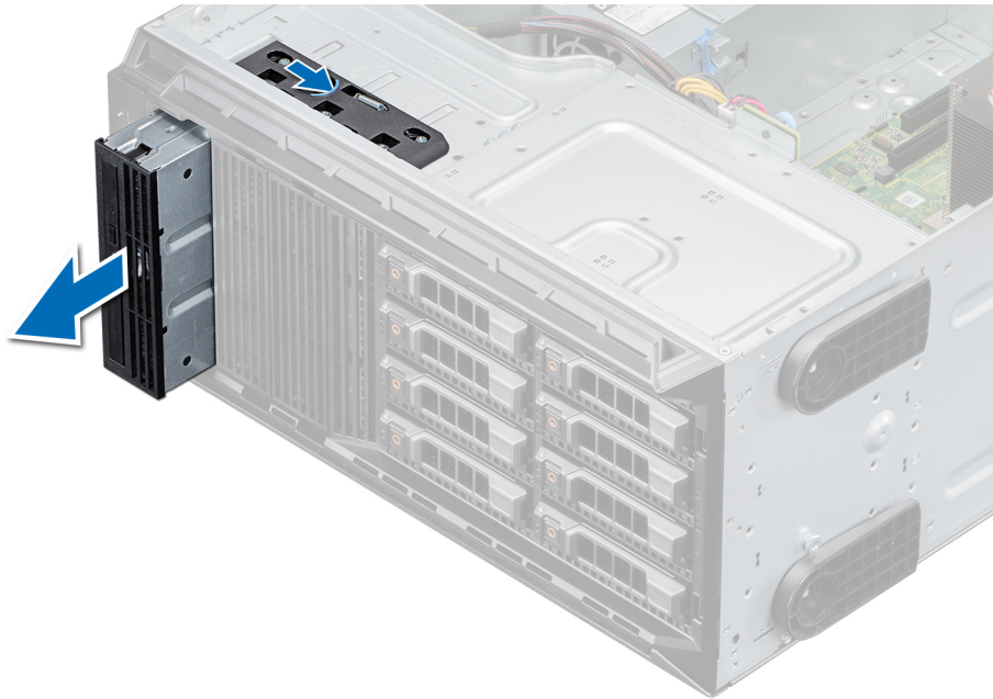
Figure 40. Removing the optical drive
