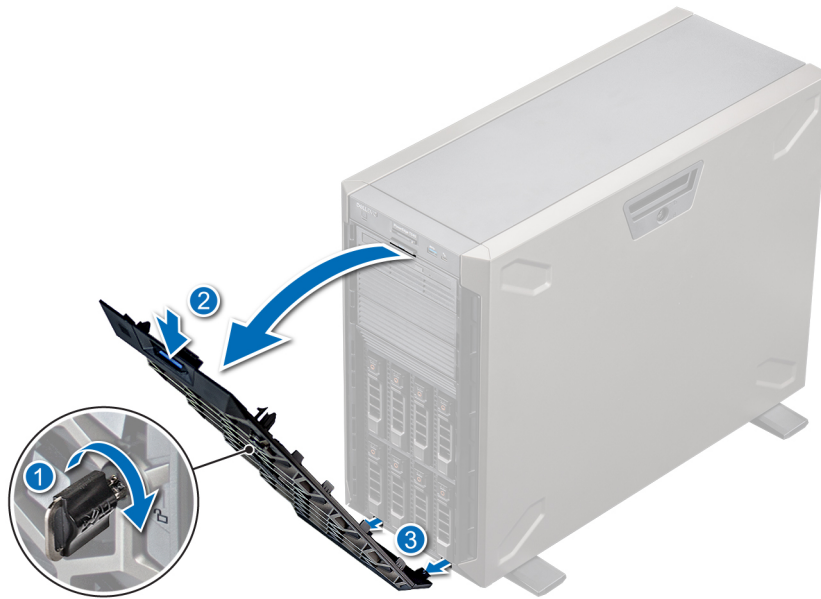
Figure 17. Removing the front bezel
