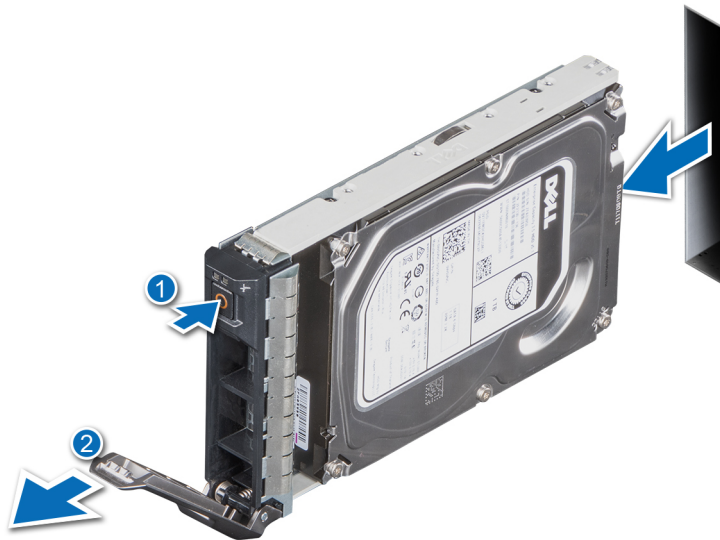
Figure 30. Removing a drive carrier
