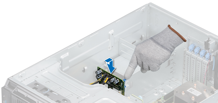
Figure 77. Installing the power interposer board
