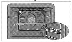
When removing tray from top oven, pull as shown in picture and hold with two hands from two sides.
