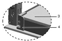
Pull the inner glass panel (3) towards yourself until it detaches from its plastic slots (4).  When reinstalling the glass panel, make sure that it is seated into the plastic slots.
