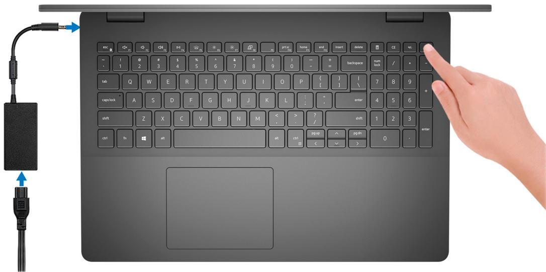
***(i)* NOTE:** To conserve battery power, the battery might enter power saving mode. Connect the power adapter and press the power button to turn on the computer.
