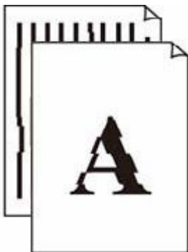
Lines Are Misaligned/Distorted
