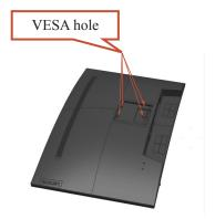
Step 5: Attach the LCD display to the wall, following the instructions in the wallmounting kit.
