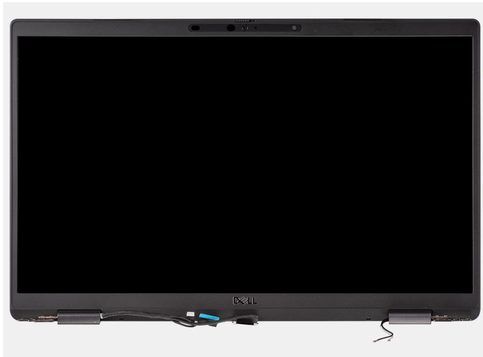
Figure 4. Display assembly with antennae cables
