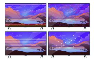
If the issue persists, define exactly what is wrong with the display. For example, mosaics and blocks, multiple lines or white dots or fixed horizontal or vertical lines.
