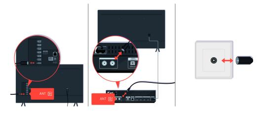
Check the antenna and input cable connections.
