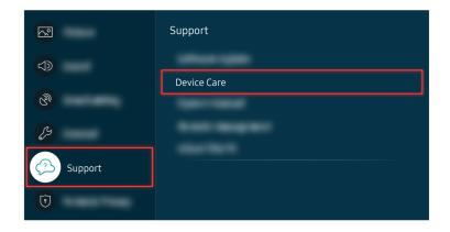
Select (a) > (a) Settings > Support > Device Care > Self Diagnosis > Signal Information to check the signal strength.
