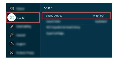
Check the volume on the screen. If a number for the TV volume is not displayed, select > Settings > Sound > Sound Output. Then, select TV Speaker.
