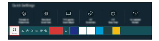
$\mbox{Go to } \mbox{ \^{o}} > \mbox{ \^{g}} \mbox{ Settings} > \mbox{ Support} > \mbox{ Device Care} > \mbox{ Self Diagnosis} > \mbox{ Sound Test to check the sound}.$
