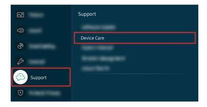
To check sound output, select (a) > (3) Settings > Support > Device Care > Self Diagnosis > Sound Test.
