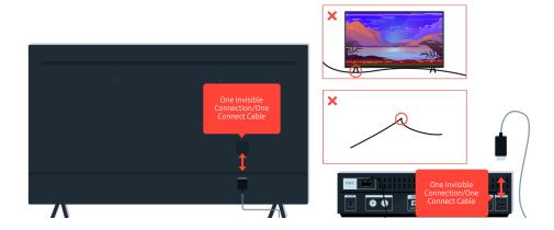
If the problem persists and if your TV uses the One Invisible Connection or One Connect Cable, disconnect and reconnect the One Invisible Connection or One Connect Cable to the TV and the One Connect Box. Ensure that the One Invisible Connection or One Connect Cable is not pinched or bent sharply.
