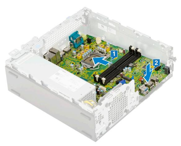
Replace the single (#6-32) screw, single (M3x5) screw and screws (5) that secure the system board to the system [1,2]. 3
