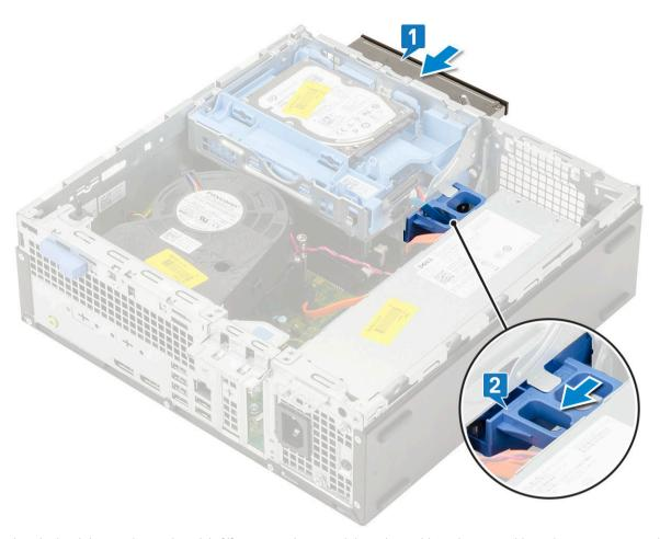
Lift the hard drive and optical module [1], connect the optical drive data cable and power cable to the connectors on the optical drive [2, 3].
