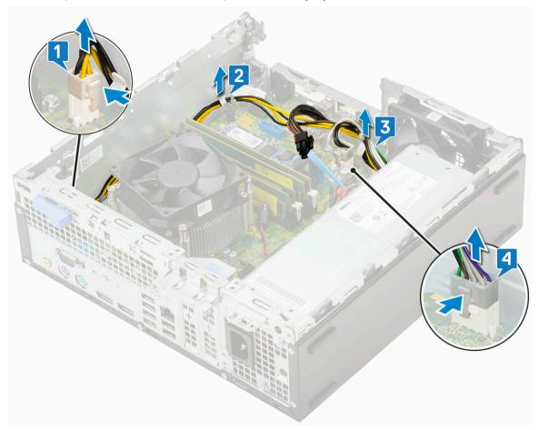
c Disconnect the system power cable from the connector on the system board [4].
