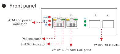
Attention1: This product must be well grounded against lightning , please use better than 20# cable to connect the grounding terminal and ground.
