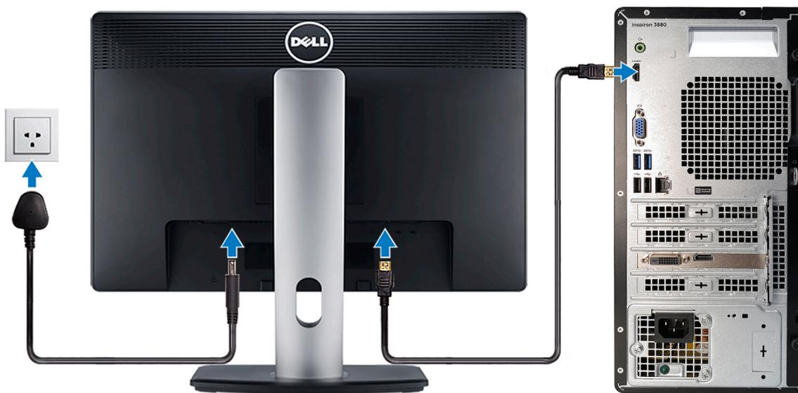
**NOTE:** If you ordered your computer with a discrete graphics card, the HDMI and VGA ports on the back panel of your computer are covered. Connect the display to the discrete graphics card.
