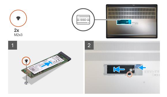
1. Place the M.2 2280 SSD onto its slot on SSD carrier.
