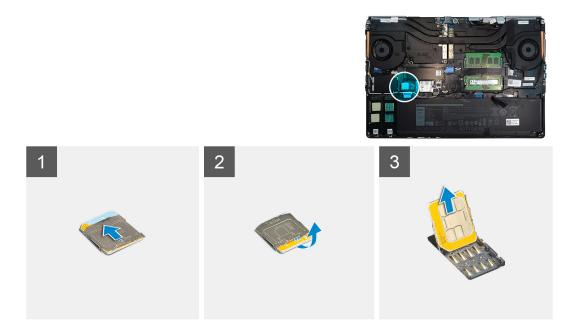
1. Gently slide the SIM card cover towards the left side of the system to unlock the SIM card cover.
