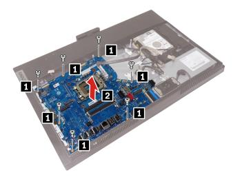
**Note:** The failing system board must be returned with a microprocessor socket cover to protect the pins during shipping and handling.
