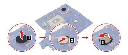
Note: After installing a new coin-cell battery, reset the system date and time in the UEFI BIOS menu.
