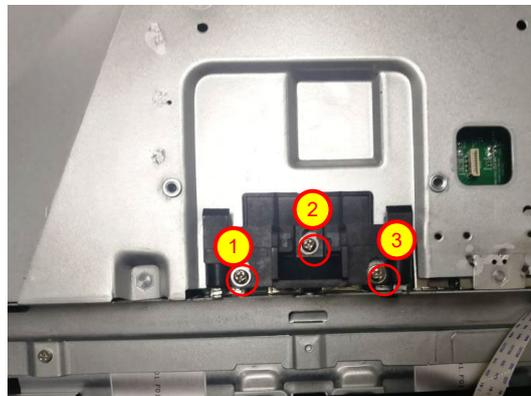
Use a Philips-head screwdriver to remove 3 screws for unlocking the latch.
