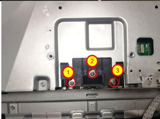
Use a Philips-head screwdriver to lock 3 screws to unlocking the latch.
