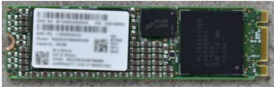
Figure 4. Disque SSD M.2 (380/F)
