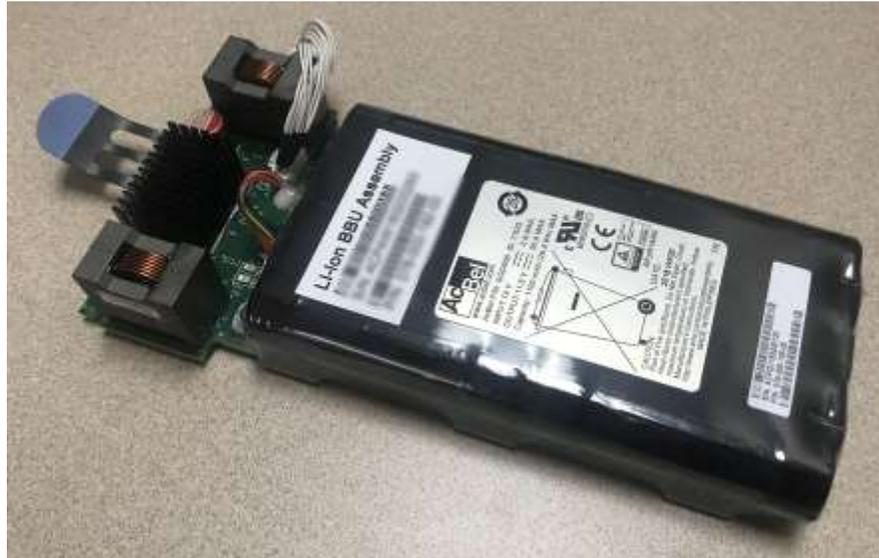
Figure 15. Bloc-batteries de secours (480/F, 680/F, 880/F)
