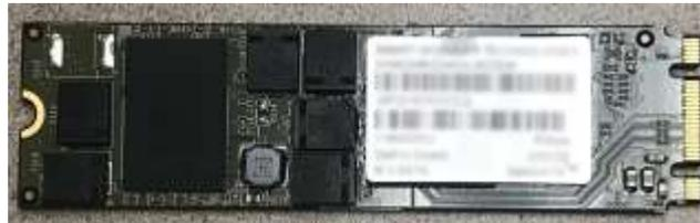
Figure 13. Disque SSD M.2 SATA (480/F, 680/F, 880/F)
