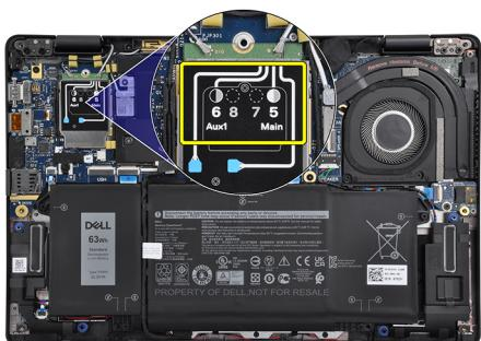
2. Loosen the single (M2x2.5) screw and remove the WWAN-card bracket.
