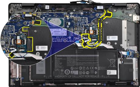
4. Replace the tweeters and palmrest antenna assembly into its slot in the palmrest assembly.
