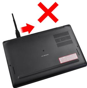
3. Pry open the left and right sides of the base cover.
