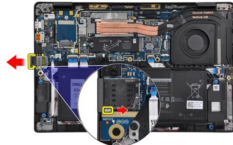
must be removed from the system before removing the system board.
