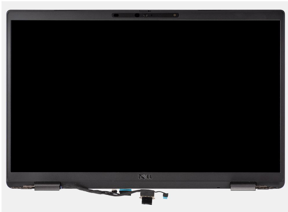
**Figure 1. Display assembly without antennae cables**
