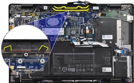
5. Replace the display cable bracket on the eDP connector on the system board.
