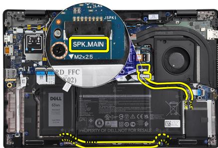
Connect the main speaker cable to the **SPK.MAIN** connector on the speaker board and route the speaker cable over the tweeter speaker cable.
