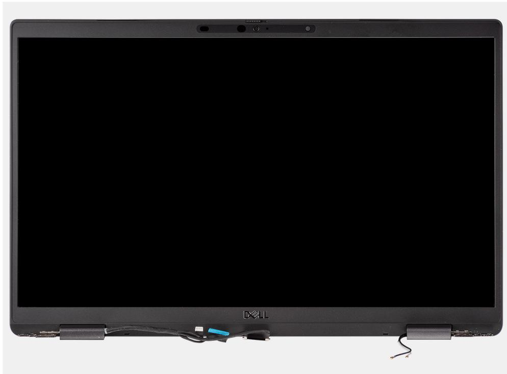
**Figure 4. Display assembly with antennae cables**
