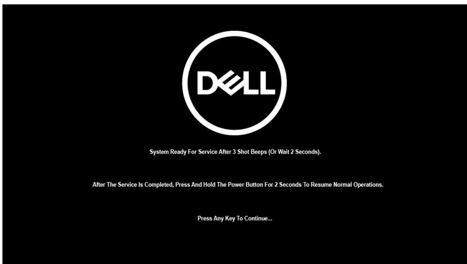
Once the system shuts down, you can perform replacement procedures without disconnecting the battery cable from the system board.
