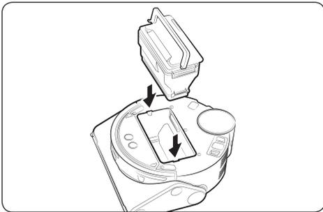
9 Attach the Dustbin to the Jet Bot. Grasp the handle and put the Dustbin into both grooves.
