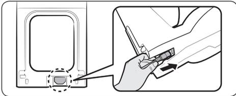
**1** Connect the provided power cord to the bottom of the Clean Station.
