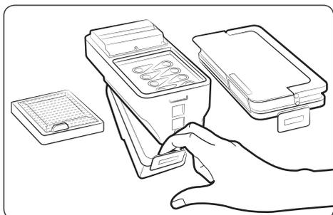
5 Unlock the transparent clip at the bottom of the Dustbin to open its Lower Cover.
