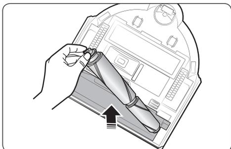
3 Lift up the left side of the brush first and then pull the brush from the groove on the right.
