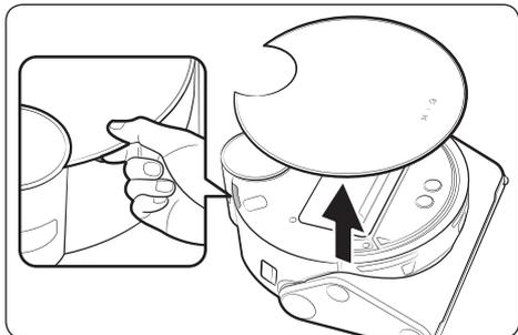
1 Detach the upper cover using the groove under the cover.
