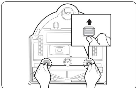
1 Push the Brush Cover Lock upward to unlock.
