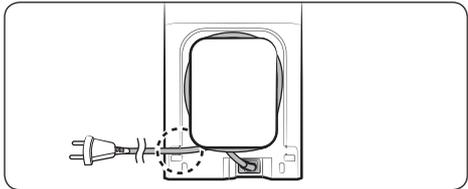
**2** Position the power cord into the fixing groove at the rear of the Clean Station.
