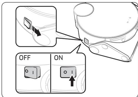
**1 Remove the yellow gasket attached to the power switch at the side of the Jet Bot and press the power switch to turn the Jet Bot on.**
