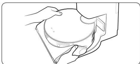
**2 Place the Jet Bot on the Clean Station manually to start charging.**
