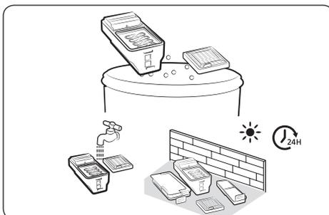
6 Remove the dust on the filter and Dustbin, clean them with water, and dry completely in the shade.
