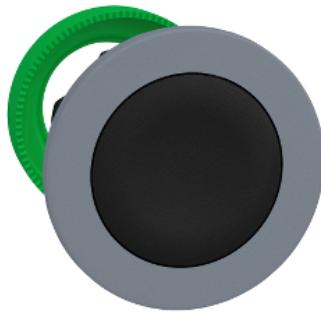
Harmony XB5, Flush mounted push button head, plastic, black, Ø30, spring return, unmarked, grey bezel
