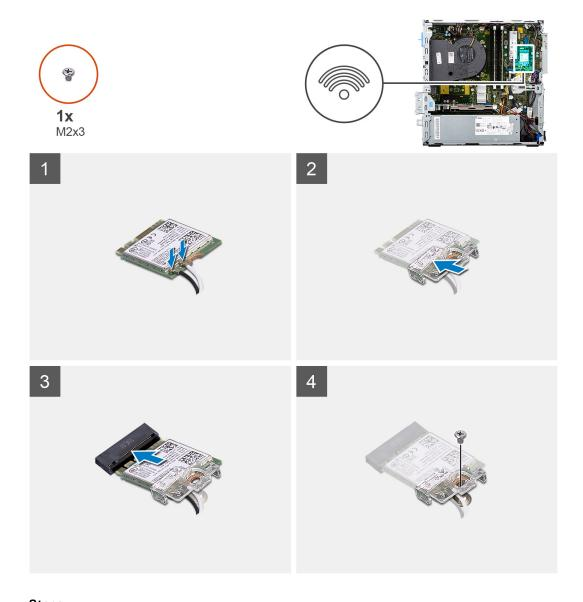
Connect the antenna cables to the WLAN card.
